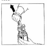
Fig 3: Grasp fittering device by head strap and pull out of case.
