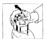
Fig 1: Push sealed opening lever upwards till seal breaks; pull locking assembly off case.
