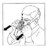
Fig 6: Position head strap and shorten if necessary.
