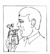
Fig 4: Bend up nose clip and insert mouthpiece (rubber flange between lips and teeth). Bite down on the two lugs.
