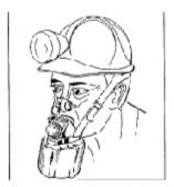
Fig 8: In case the FSR cannot be pulled out of its case (if, e.g. the case is badly dented), the FSR can still be used with the case bottom, however, with increased inhalation resistance.
